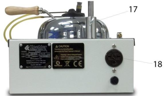
17. **Motor Support Rod Adjustment Screw.** For tightening and securing motor support rod to base assembly.
