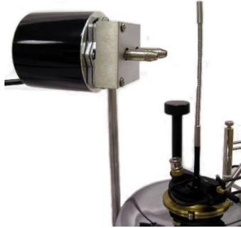
After approximately 100 hours of use, remove the motor cover and locate the two drive shafts. Place a few drops of light lubricating oil such as **3 in 1** into the bottom of each shaft and re-install the motor cover.
