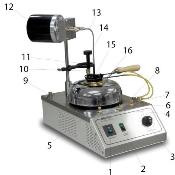
1. **Main Power Switch.** Controls power to the entire unit. Pressing the switch to the ON position will energize the instrument. Pressing the switch to the OFF position will de-energize the instrument. Switch will illuminate when in the ON position
